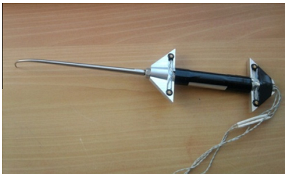
Fig. 3. A self-designed pointer to define the positions of holes in the calibration phantom.
