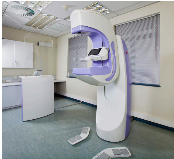
Figure 1. The Aceso dual-modality system as installed for the clinical trial, showing the acquisition workstation with iPad, a pair of foot pedals, gantry, and C-arm.
