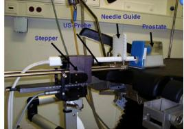
Figure 1. BiopSee system consists of personal computer with integrated US device and additional electronics to control position and orientation of US probe. Probe has custom biplane endorectal design and is placed on custom mechanical stepper. Device movement is tracked by 2 encoders with resolution of 0.1 mm and 0.1 degree.
