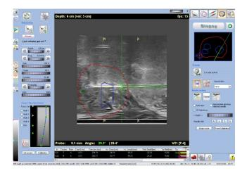
**Figure 4.** Biopsy needle inserted under continuous longitudinal US guidance. US image was overlaid by organ and lesion contours and planned needle trajectory to enable real-time navigation so that deviations from target were immediately visible on screen and could be corrected. After each biopsy, needle position and orientation data were stored for documentation.
