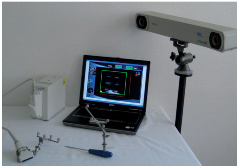
Figure 9. Components for sononavigation: ultrasound device with navigated scanner (left), navigated pointer, PC with custom software (center), and Polarix coordinate tracker (right).
