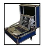
Figure 1. TelaVet 1000 PC based scanner in its hard sided case.
