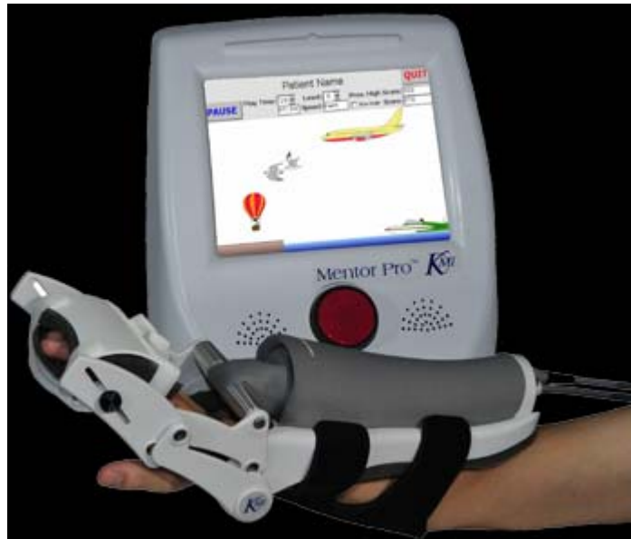
Figure 4: The Hand Mentor™ from Kinetic Muscles Inc. is a rehabilitative hand exoskeleton used for therapeutic treatment [25].
