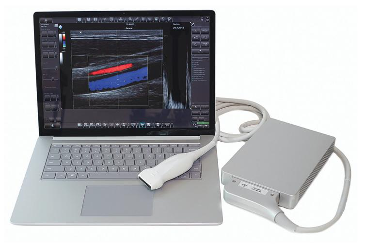
elemed offers the tool for real-time RF data access (B-mode + RF Data) acquisition - RF Data Control and the packages for data processing, implemented in MATLAB, Python and LabView environments.
